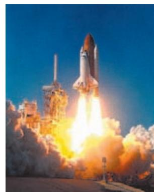
**Figure 19.15 | Blastoff of the space shuttle.** The large negative heat of formation of  $Al_2O_3$  provides power to the solid-state booster rockets that lift the space shuttle from its launch pad. (NASA)
