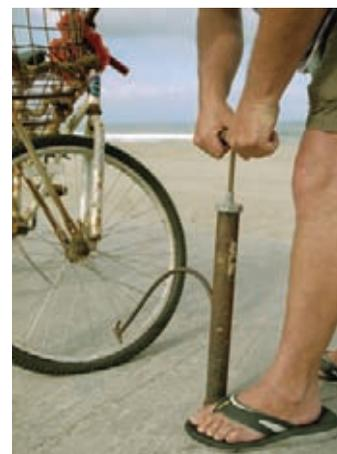
**Figure 19.2 | Work being done on a gas.** When a gas is *compressed* by an external pressure,  $w$  is positive because work is done on the gas. Because  $V$  decreases when the gas is compressed, the negative sign assures that  $w$  will be positive for the compression of a gas. (Lawrence Manning/Corbis Images)
