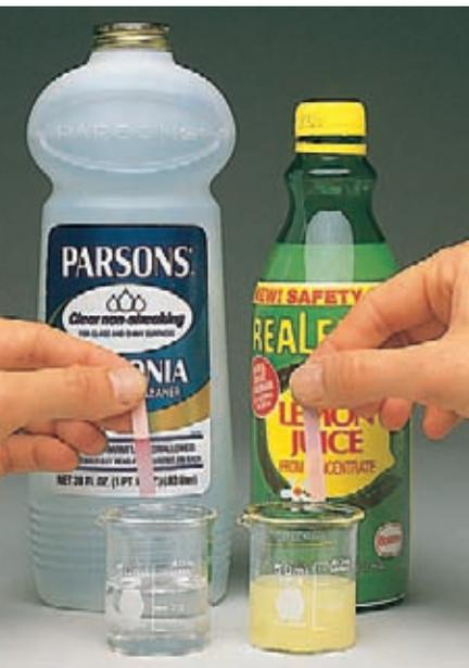
**Figure 5.9 | An acid–base indicator.** Litmus paper, a strip of paper impregnated with the dye litmus, becomes blue in aqueous ammonia (a base) and pink in lemon juice (which contains citric acid). (Ken Karp)
