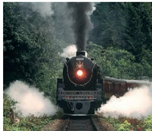
**Figure 19.1 | Expanding gases can do work.** In a steam engine, such as the one powering this locomotive, heat is absorbed by water to turn it into high temperature, high pressure steam ( $q$  is positive). The steam then expands, pushing pistons and causing the locomotive to move. In the expansion, the steam does work and  $w$  is negative. (Richard A. CookeIII/Stone/Getty Images)
