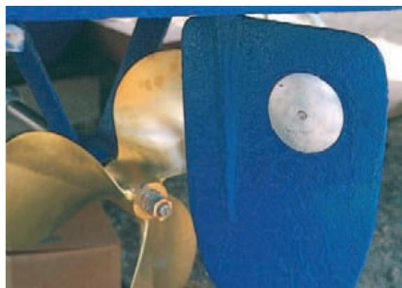
Figure 2 **Cathodic protection.** Before launching, a shiny new zinc anode disk is attached to the bronze rudder of this boat to provide cathodic protection. Over time, the zinc will corrode instead of the less reactive bronze. (The rudder is painted with a special blue paint to inhibit the growth of barnacles.) (Courtesy James Brady)
