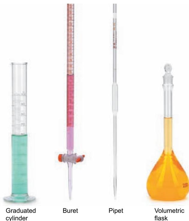
**Figure 2.6 | Common laboratory glassware used for measuring volumes.** Graduated cylinders are used for measuring volumes to the nearest milliliter. Precise measurements of volumes are made using burets, pipets, and volumetric flasks. (*Andy Washnik*)
