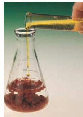
**Figure 18.1 | Silver chromate.** When sodium chromate is added to a solution of silver nitrate, deep red-brown “insoluble” silver chromate,  $\text{Ag}_2\text{CrO}_4$ , precipitates. (Michael Watson)
